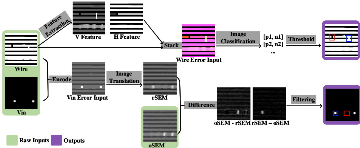
Fig. 2. Pipeline of the proposed approach. rSEM: reconstructed SEM image. oSEM: original SEM image. Red bounding boxes: "open" of wires or "miss" vias. Blue bounding boxes: "short" of wires or "extra" vias
