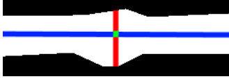
Fig. 3. For a given pixel(green), the horizontal and vertical extension values are defined as the length of blue and red lines, respectively.
