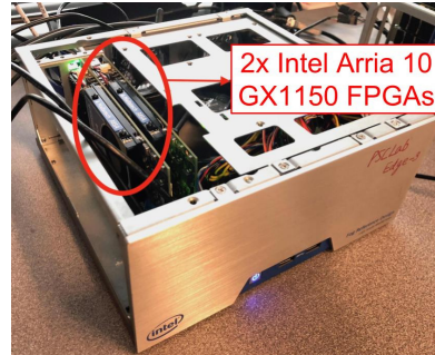
Figure 1: An Intel Fog Reference Design unit hosting two Nallatech 385A FPGA Acceleration Cards.
